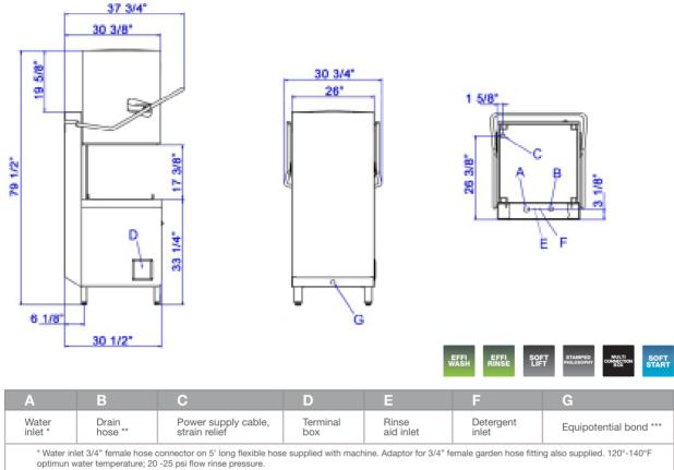
\*\* Drain 5' long, 1/2" I.D. flexible hose. Maximun 26 3/4" drain height permites indirect connection to drain pump.\*\*\* Protection from dangerous potential differences
