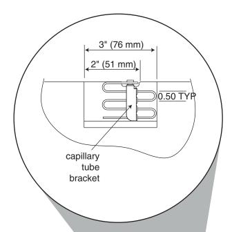
Thermostat: hand bend cap tube end as shown
