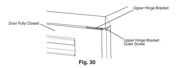
20) Check the door operation to assure it opens and closes properly. Note: Hold door at 45° angle from closed position and release. Door should close on its own. If not, adjust hinge bracket.
