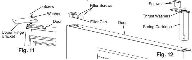
9) Clear foam from the spring cartridge hole to allow for spring cartridge installation. See Fig. 13. Install the spring cartridge in its new location. Reinstall the filler cap and filler screws on the opposite side of the door.
