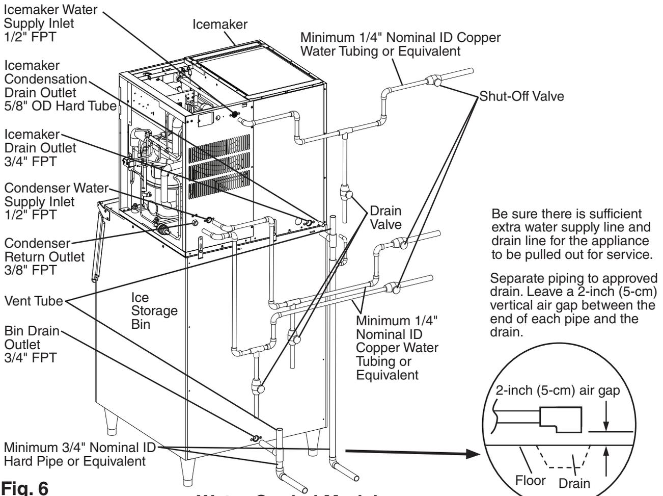
Be sure there is sufficient extra water supply line and drain line for the appliance to be pulled out for service.
