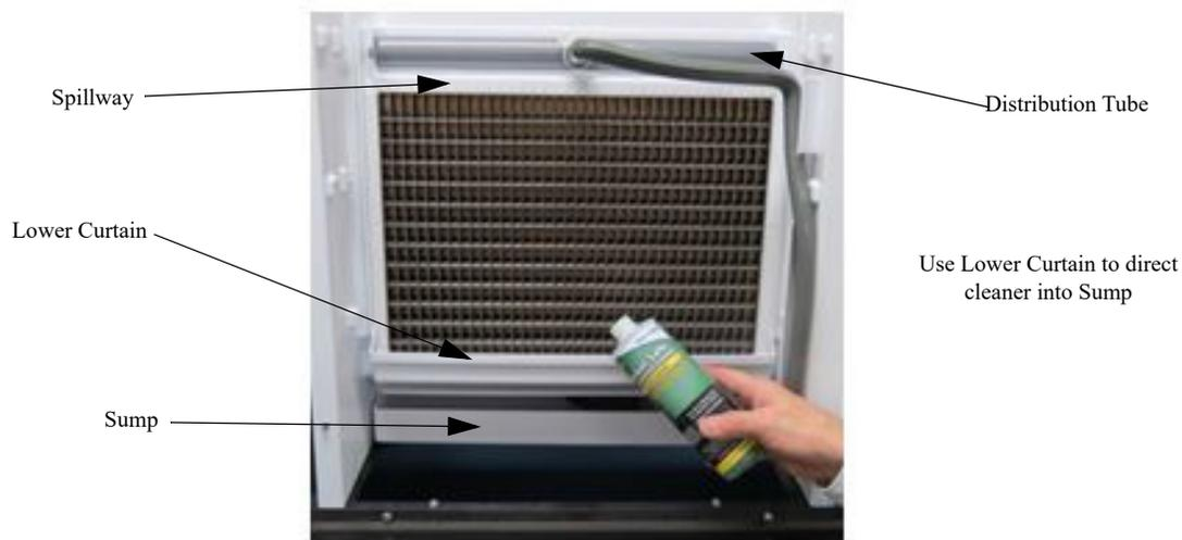
10. The machine will remain in the WASH cycle for 15 minutes (cycle may be shortened after a minimum of 5 minutes if CLEAN button is depressed).
