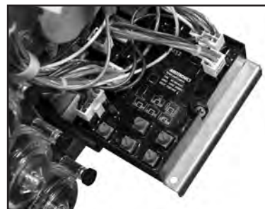
Circuit board slides out for easy access
