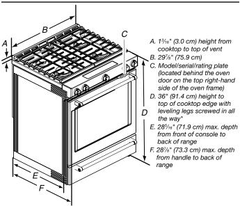
**IMPORTANT:** Range must be level after installation. Follow the instructions in the "Level Range" section. Using the cooktop as a reference for leveling the range is not recommended.
