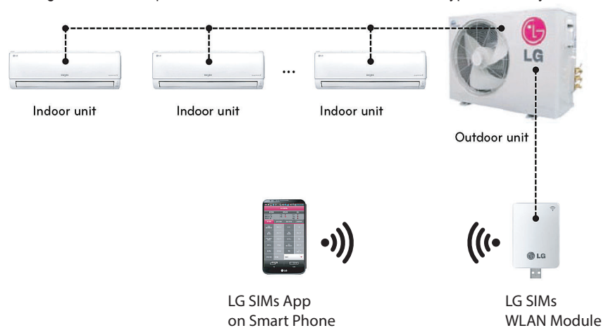
Figure 139: Example of a SIMS WLAN Module Used with a Typical DFS System.
