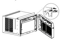
Attach the front grille to the cabinet by inserting the tabs on the grille into the slots on the front top of the cabinet.
