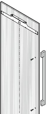
Only use countersunk screws for handle mounting.
