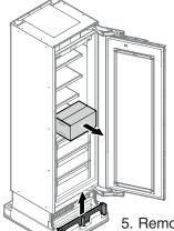
4. Remove the box with mounting parts.
