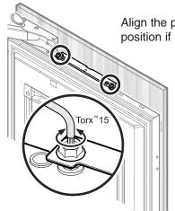
Align the panel in its vertical position if necessary.
