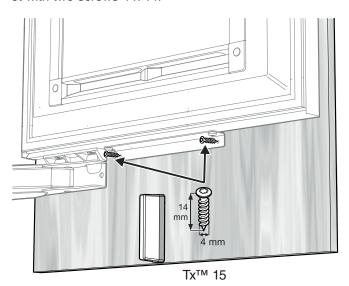
Insert the panel supports into the support strips between panel and appliance door and screw into place with two screws M6 x 12 each.
