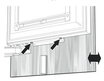
Fasten the panel through the bottom attachment bracket with two screws  $4 \times 14$ .
