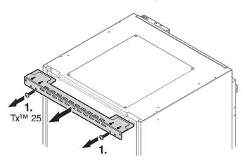
1. Remove the anti-tipping bracket. The screws are no longer needed.
