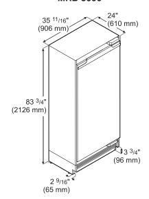
Stated minimum height dimensions include when the levelled feet are fully inserted. Width will increase by 1/4" (6.5 mm) when mounting strips are installed.
