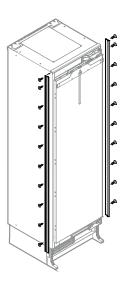
Apply the appliance cover strips to the left and right front edge of the appliance housing, align in height with the top profile and screw into place. The strip is transparent so the designed mounting holes on the appliance housing are visible.
