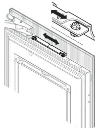
Align the panel horizontally with the long holes in the attachment bracket.
