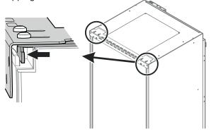
Adjustment of the anti-tipping bracket for use in a 25" deep recess
