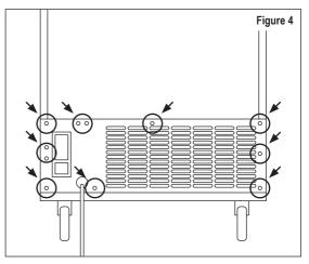
Use a commercial condenser coil cleaner, available from any kitchen equipment retailer. Brush the condenser fins from top to bottom, not side to side. After cleaning, straighten any bent condenser fins with a fin comb.
