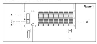
The control panel and display are located at the bottom rear of the unit, next to the main power switch.
