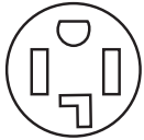
4-wire receptacle (14-30R)
