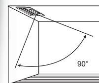
Operate the remote controller in the area where signal is received, and beep is heard.
