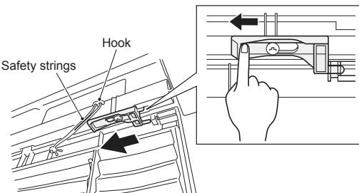
2. Install the intake grille by following the removal procedure in reverse.
