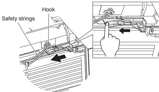
2. Install the intake grille by following the removal procedure in reverse.
