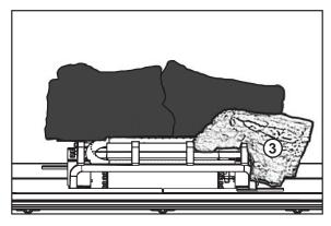
C. Place log #3 onto the far right locating stud located on the front deflector.
