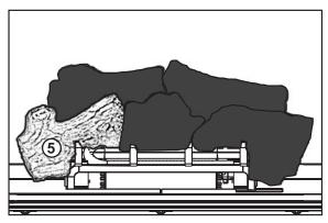
**E.** Place log #5 onto the far left locating stud located on the front deflector.
