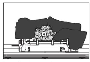
**D.** Place log #4 onto the two center locating studs on the front support.
