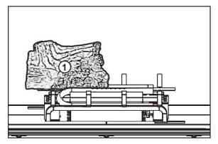
A. Place the left middle log #1 onto the locating stud on the middle log support. Make sure the hollow on the underside of the log is over the bend tab.
