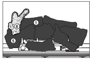
H. Place the pin in log #8 into the locating hole on log #1 and rest the bottom of the log on log #5.
