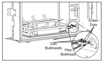
B. Connect the pilot electrode leads to the bulkhead matching the 1/4" flag with the 1/4" bulkhead spade and the 3/16" flag with the 3/16" spade.
