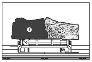
B. Slide log #2 from right to left on the middle log support creating a tight fit between logs #1 and #2. Make sure the hollow on the underside of the log is over the bend tab.
