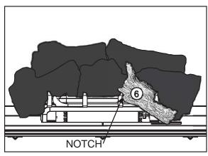
**F.** Place the notch on log #6 onto the third grate.
