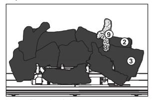
I. Place the pin in log #9 into the locating hole on log #2 and rest the bottom of the log #3.
