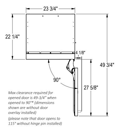
**PLEASE NOTE:** When installing column adjacent to wall, a 2" clearance is required if door opens towards the wall
