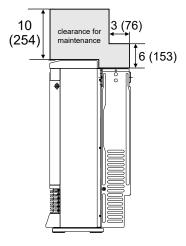
Clearances to access the furnace during servicing are 10 in. (254 mm) from the sides, 40 in. (1 m) from the front, and the area shown above the furnace in the figure to the left.
