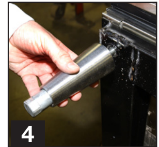
4 Thread leg into cabinet bottom frame rail.
