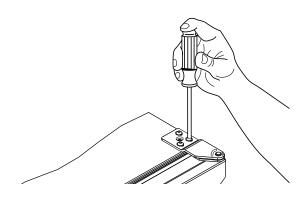
3. Remove door by tilting forward and lifting door off bottom hinge. Retain shoulder washers; they will be reused.
