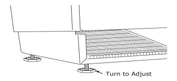
3. Confirm the unit is level after each adjustment and repeat the previous steps until the unit is level.
