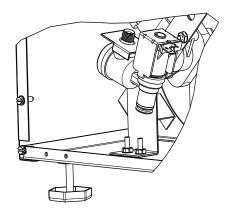
4. Break away filler feature in bushing with flat screwdriver.
