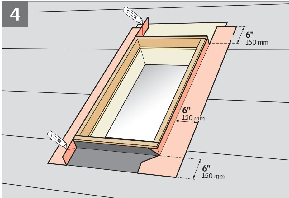
**ENGLISH:** Wrap the sides and the corners of the skylight curb with VELUX adhesive skylight underlayment and create water-shedding laps over roofing underlayment.
