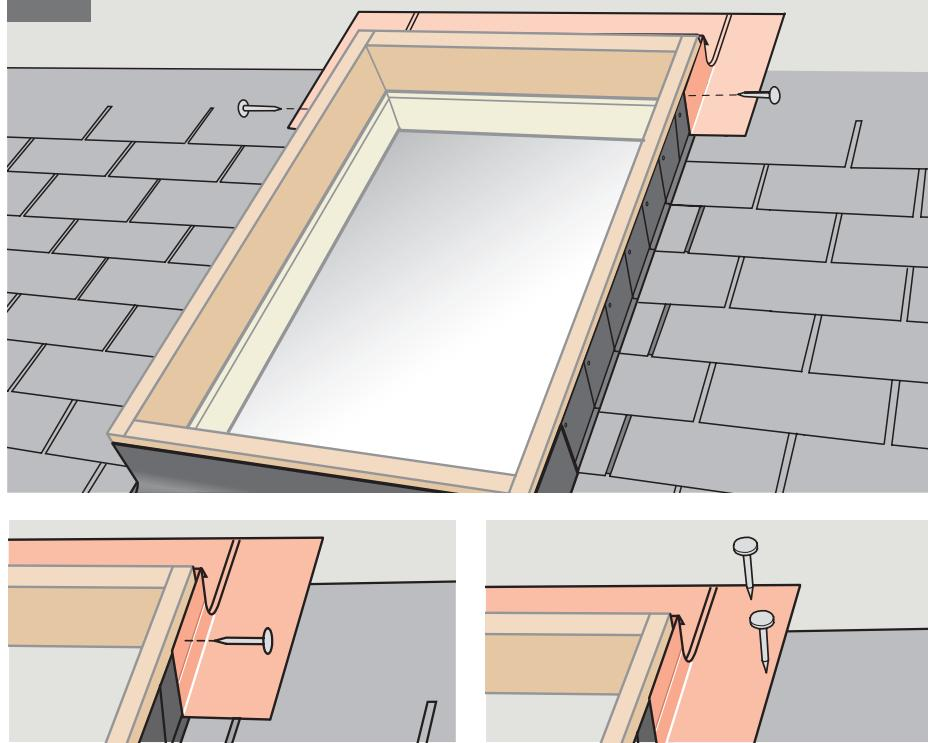
**ENGLISH:** Install and attach saddle flashing to curb or to roof with roofing nails as shown.
