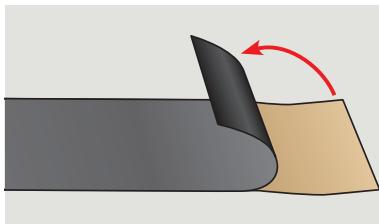
**ENGLISH:** To ensure waterproofing, skylight curbs shall be completely wrapped in VELUX adhesive skylight underlayment as indicated. Underlayment must be applied before installing the flashing. Remove existing roofing underlayment around the rough opening as shown.
