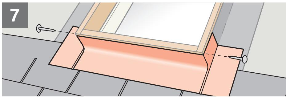
**ENGLISH:** Position and attach the sill flashing section to curb or to roof with roofing nails. Avoid exposed nails as shown.
