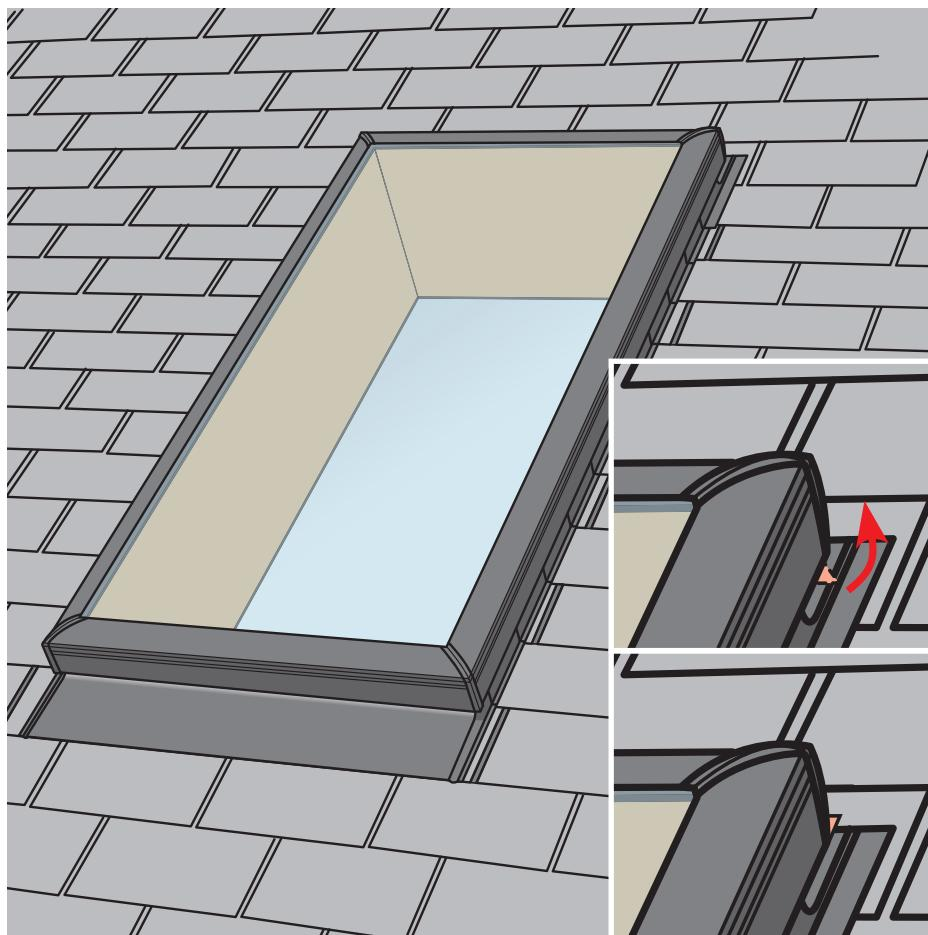
**ENGLISH:** When installing the skylight on a curb with a height of 3 1/2" (90 mm), bend the visible part of the saddle flashing as shown for extra protection.
