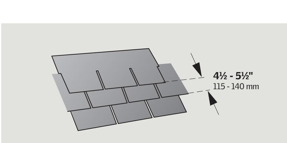
**ENGLISH:** For use with thin roofing materials with exposures between  $4\frac{1}{2}$ " (115 mm) and  $5\frac{1}{2}$ " (140 mm).
