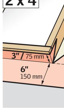
**ENGLISH:** Wrap the bottom and the corners of the skylight curb with the underlayment and create water-shedding laps over roofing underlayment.
