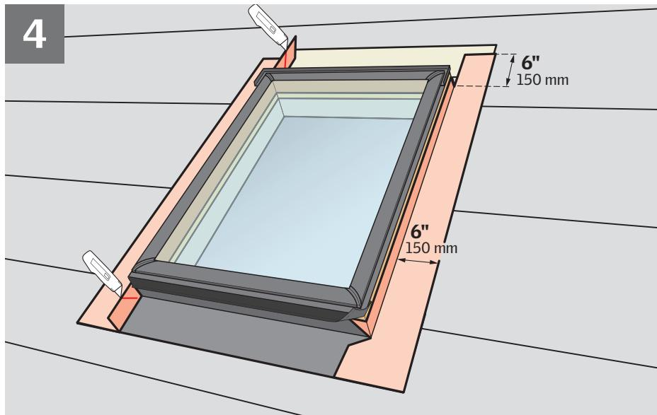
**ENGLISH:** Wrap the side frames and corners of the skylight with VELUX adhesive skylight underlayment and create water-shedding laps over roofing underlayment.
