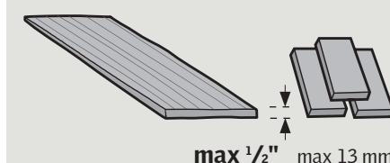
**ENGLISH:** EDL can also be used for cedar shingles and slates (max thickness  $1/2$ " (13 mm)). In this case, download specific installation instructions for flashing EDL for roofing material cedar shingles and slates or contact your VELUX sales company.
