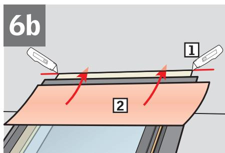
**ENGLISH:** To allow for proper drainage, interweave VELUX adhesive skylight underlayment as shown in **6a** for new construction applications. For retrofit applications, interweave VELUX adhesive skylight underlayment as shown in **6b**.
