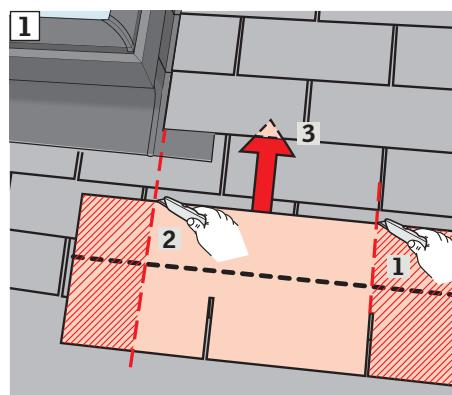
**ENGLISH:** For best installation appearances, exposed sill flashing section and saddle flashing corners can be covered with a cosmetic shingle.
