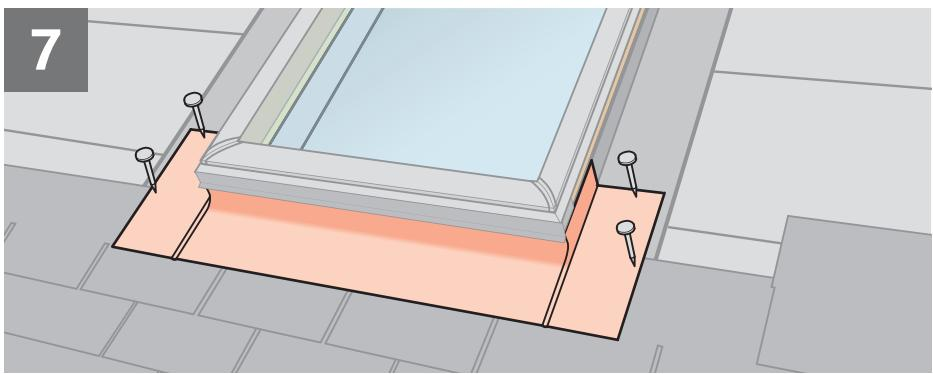
**ENGLISH:** Position sill flashing section tightly to the bottom frame and attach it with roofing nails as shown.
