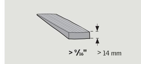
**ENGLISH:** EDL cannot be used for cedar shakes and slates thicker than  $9/16$ " (14 mm). In this case, see installation instructions for flashing EDW (for profiled roofing materials).
