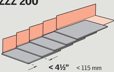
**ENGLISH:** For exposures less than  $4\frac{1}{2}$ " (115 mm) or greater than  $5\frac{1}{2}$ " (140 mm), a supplementary VELUX step flashing kit ZZZ 200 may be required.
