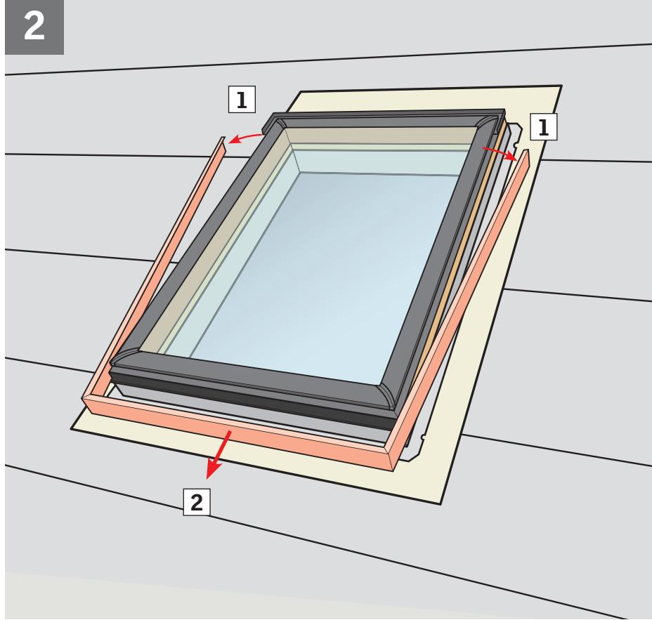
**ENGLISH:** To properly install VELUX adhesive skylight underlayment, remove cladding as shown.
