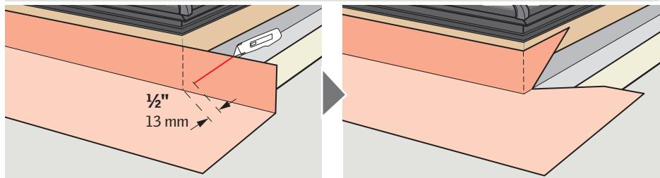
**ENGLISH:** To ensure waterproofing, skylight frames should be completely wrapped in VELUX adhesive skylight underlayment supplied with the flashing. This underlayment must be applied before installing the flashing.
