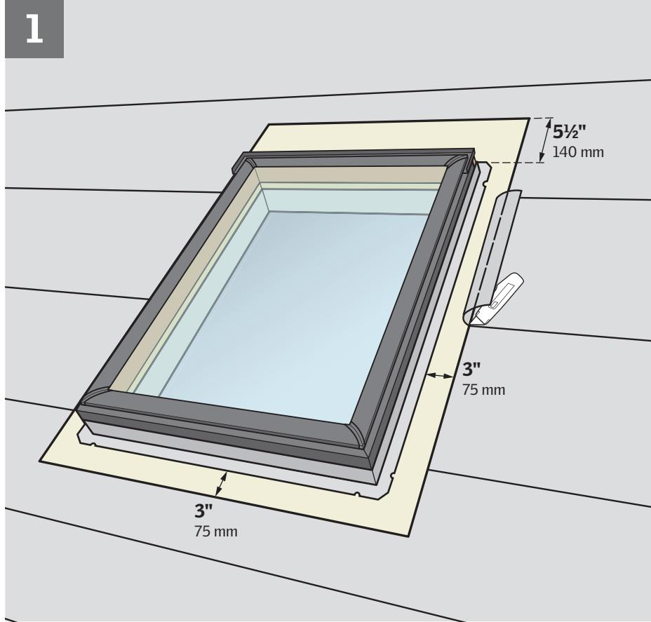
**ENGLISH:** Remove existing roofing underlayment around the rough opening as shown.
