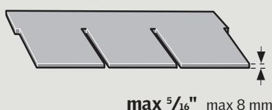
**ENGLISH:** EDL is designed for thin roofing materials (max thickness  $5/16$ " (8 mm)).
