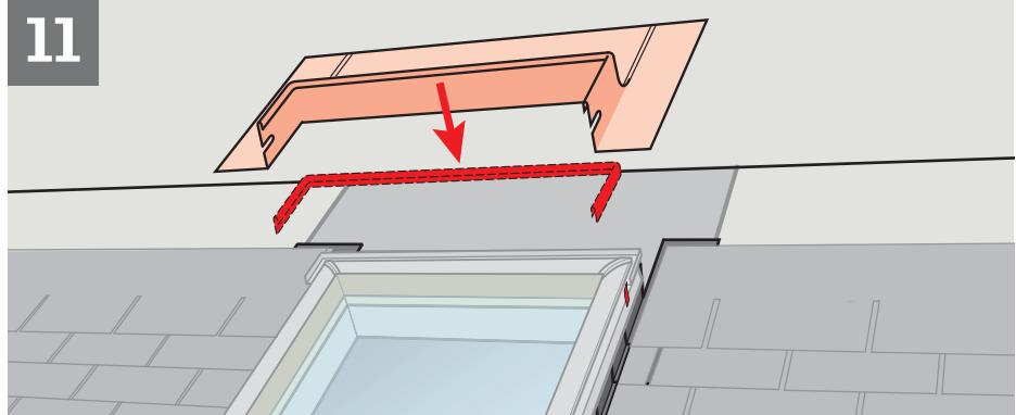
**ENGLISH:** Install saddle flashing. Determine use of extension piece: use it if the saddle flashing is lifted up by the underlying roofing material and remove it if the saddle flashing fits tightly over the skylight.
