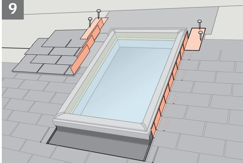
**ENGLISH:** Interweave step flashing pieces with roofing material and fasten them to roof with roofing nails. If necessary, cut the top step flashing pieces as indicated.
