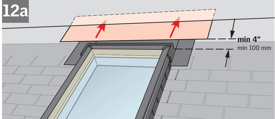
**ENGLISH:** To allow for proper drainage, interweave roofing underlayment as shown in 12a for new construction applications. For retrofit applications, interweave roofing underlayment as shown in 12b.
