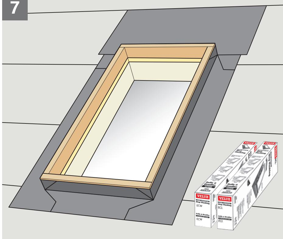
**ENGLISH:** For thin roofing materials, use flashing ECL. ECL is designed for roof pitches 10° - 60° (2:12 - 21:12).
