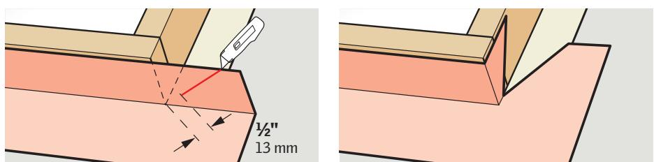
**ENGLISH:** To ensure waterproofing, skylight curbs shall be completely wrapped in VELUX adhesive skylight underlayment as indicated. Underlayment must be applied before installing the flashing. Remove existing roofing underlayment around the rough opening as shown.
