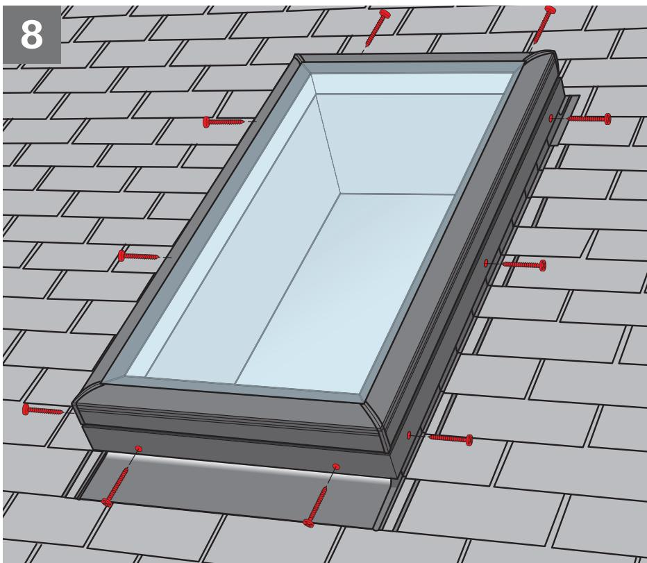
**ENGLISH:** Center the skylight on top of the curb and secure with #8 1¾" (4.2 x 45 mm) pan head stainless steel screws provided. Screws will penetrate the curb by at least ¾" (19 mm).
