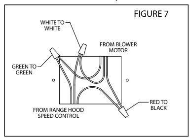
Push wires back into the wiring compartment and reinstall the wire-box cover and gasket as shown below.
