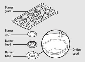
2. Using a 9/32" or 7 mm nut driver remove the top burner orifices. These may be accessed through the opening in the burner base.
