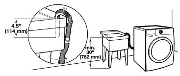
Minimum capacity: 20 gal. (76 L). Top of laundry tub must be at least 30" (762 mm) above floor; install no higher than 96" (2.44 m) from bottom of washer.
