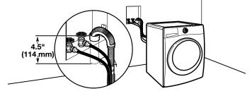
See requirements for floor standpipe drain system.
