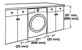
All dimensions show recommended spacing allowed, except for closet door ventilation openings which are the minimum required.
