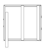
Place charcoal filter on backside of filter. And place filter brackets over charcoal filter and secure in place by tucking each end of bracket under the filter frame. Reinstall filter.
