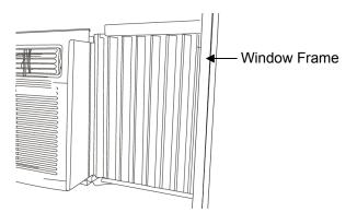
NOTE: When choosing your window make sure the power supply cord is within 4 feet of a grounded 3-prong outlet.
