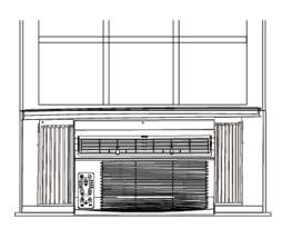
NOTE: Check that the air conditioner cabinet is tilted back about 1  $\frac{1}{8}$ " to 1  $\frac{1}{2}$ ", which should be about 3-4 degrees downward to the outside. After proper installation, condensation should not drain from the overflow drain hole during normal use, correct slope or otherwise.
