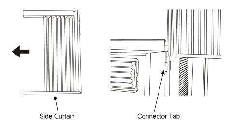
5. Insert the top and bottom of the curtain housing to the top curtain and bottom curtain channel.
