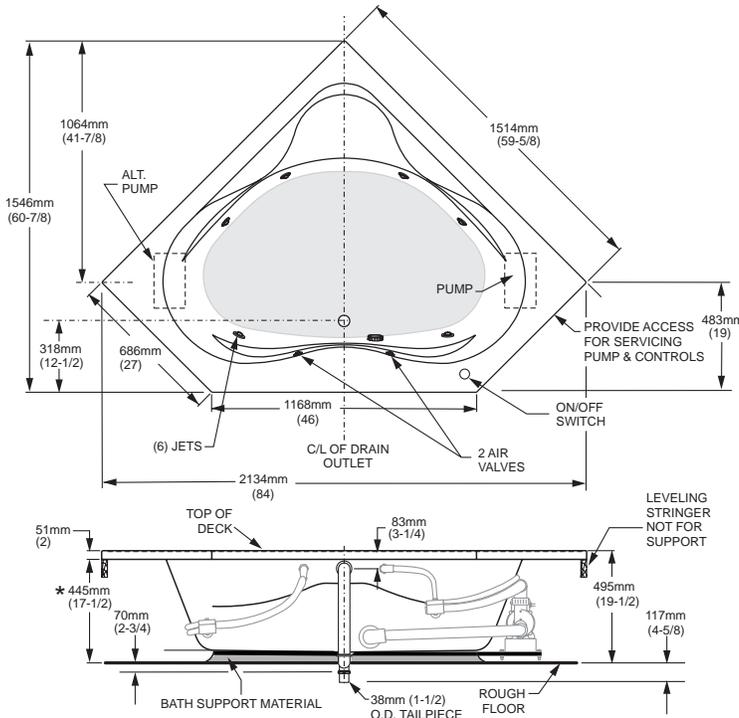
\* **NOTE:** If the optional apron (PN 0730.121) is to be used with this tub, the stringer height must be referenced from the finished floor.
