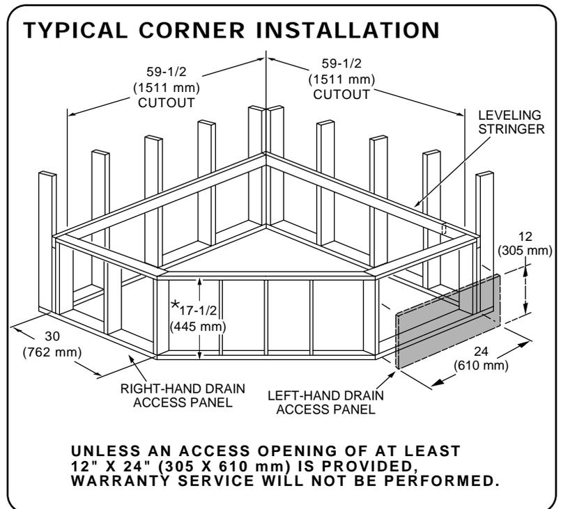
\* NOTE: If the optional apron (PN 0730.121) is to be used with this tub, the stringer height must be referenced from the finished floor.
