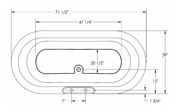
These dimensions are for reference only, and can vary +/- 1/4". If exact measurements are required, please use the actual tub to be installed.
