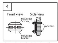
Push anchors into the drilled holes until flush with the wall surface. Fasten mounting bracket to the wall with mounting screws.
