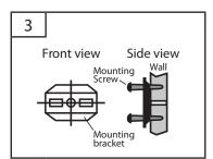
Drill 1/4" holes in drywall through the mounting screw holes. If attaching onto a wood wall, fasten mounting bracket directly to the wall with screws without pre-drilling the holes.
