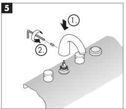
Install the spout (1) to the spout adapter over the diverter. Tighten the set screw (2) with the enclosed 3 mm allen wrench.
