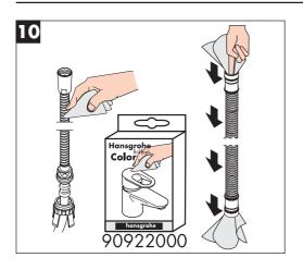
Use the enclosed cleaning towelette to thoroughly clean the outer Secuflex<sup>TM</sup> hose.
