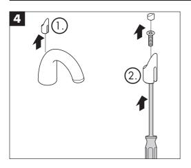
Remove the diverter knob from the spout (1). Use a small screwdriver to push the screw and screw cover from the diverter knob (2).
