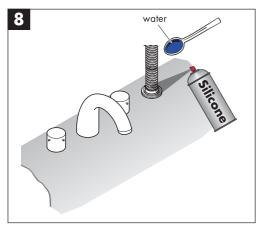
Lubricate the handshowr mount and outer Secuflex<sup>TM</sup> hose with spray silicon lubricant or with a tablespoon or so of water.
