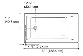
No change in measurements if connected with required drain illustrated. (K-7272)
