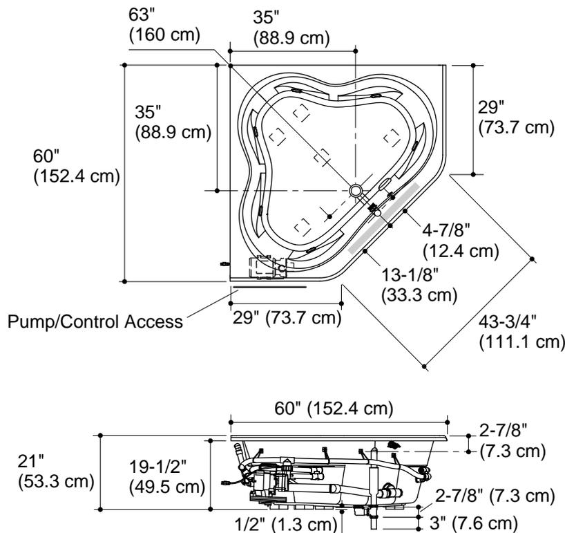
No change in measurements if connected with drain illustrated. (K-11677 or K-11677M)
