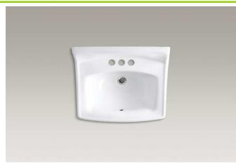
The wall-mount lavatory shall be made of vitreous china. Lavatory shall be with overflow or without overflow. Lavatory shall be 20-3/4" (527 mm) in length, and 18-1/4" (464 mm) in width. Lavatory shall be for 4" (102 mm) centers and drilled for concealed arm carrier. Lavatory shall have hanger. Lavatory shall be available with optional soap dispenser hole on left (-L) or right (-R).
