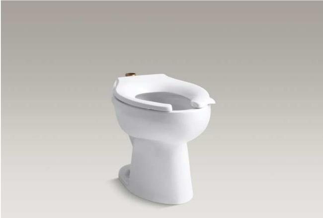
The elongated bowl shall be 10" (254 mm) or 12" (305 mm) rough-in with a 1-1/2" top spud. Bowl shall be made of vitreous china. Bowl shall be 1.6 gpf (6 lpf). Bowl shall have 11-3/8" (289 mm) x 10-3/8" (264 mm) water area. Bowl shall have 2-1/4" (57 mm) passageway. Bowl shall have bedpan lugs (-L). Bowl shall be 26" (660 mm) in length, 14-1/2" (368 mm) in width, and 17-1/2" (445 mm) in height.
