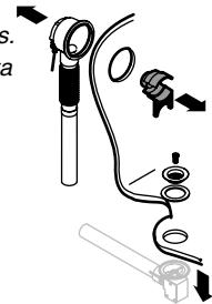
**16** Apply silicone sealant to the gaskets.
