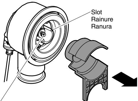
**IMPORTANT!:** Make sure the center of the push button is centered in the opening.
