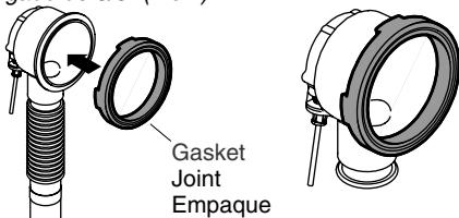
If "A" is less than 1/4" (6 mm): install the thick gasket, 9/16" (1.4 cm).
