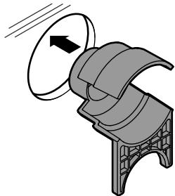
**4** Dry fit drain ell and secure with retainer.
