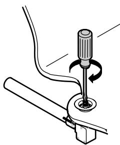
**20** Loosely install the overflow flange.
