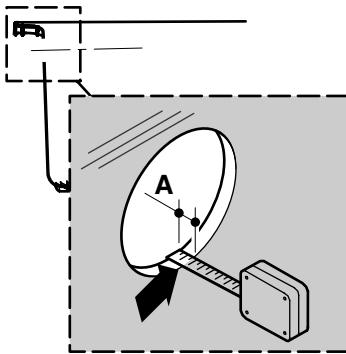
**2** If "A" is 1/4" (6 mm) or greater: install the thin gasket, 3/8" (1 cm).
