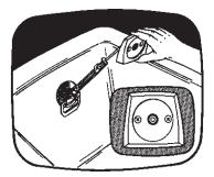
12 Insert the lift assembly into the overflow. Tighten the overflow hood to the overflow ell with the two screws provided. Refer to inset.
