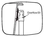
**7** Align the overflow ell with the overflow hole in the bath.
