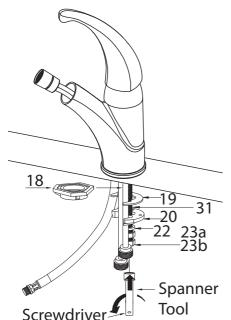
Install the faucet extender (18), rubber u-washer (19), and metal u-washer (20) on the mounting pipe (31) until it touches the base of the countertop. Place metal o-ring (22) and thread metal nut (23a) onto the mounting pipe (31) and tighten with the provided spanner until snug.
