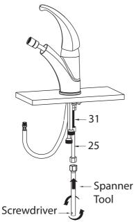
Secure on extending pipe (25) on the mounting pipe (31) and tighten with the provided spanner until snug
