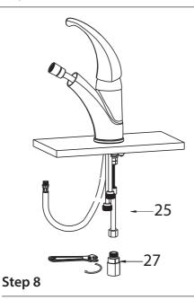
Secure the check valve assembly (27) onto the extending pipe (25). Tighten with an adjustable wrench until snug
