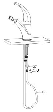
Secure the end of the hose (10) onto the check valve assembly (27) and tighten with an adjustable wrench until snug
