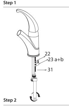
Remove the metal o-ring (22) and metal nuts (23a and 23b) from the end of the mounting pipe (31)
