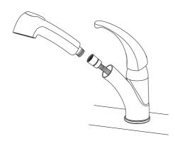
Secure the spray head (9) onto the hose (10) and hand-tighten only
