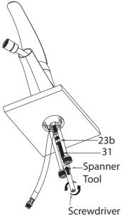
Place metal nut (23b) on the mounting pipe (31) and tighten with the provided spanner until snug underneath the countertop
