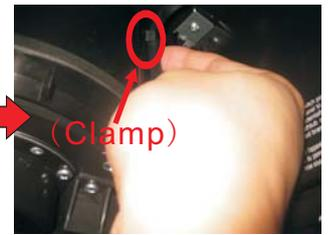
Pull out the lead wire from Casing clamp
