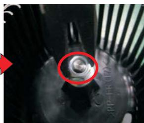
Remove the blade fixing nut
