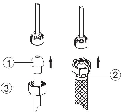
Make connections to water lines. Use 1/2" I.P.S. faucet connections (2) or use supply line coupling nuts (3) with 3/8" O.D.ball-nose riser (1). Use wrenches to tighten connections. Do not overtighten.
