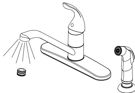
**Important:** After installation is completed, remove aerator. Turn on water supply and allow both hot and cold water to run for at least one minute each. While water is running, check for leaks. Replace aerator.
