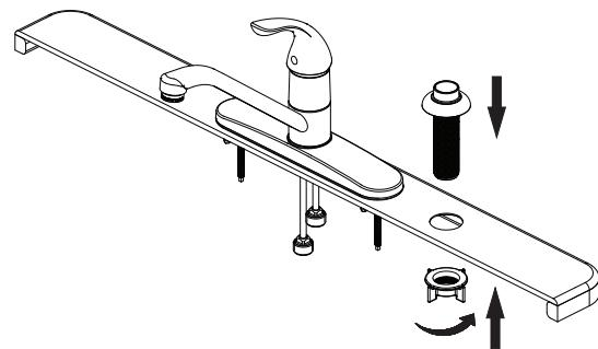
Insert spray support through far right hole on escutcheon. Screw nut onto shank and hand tighten.
