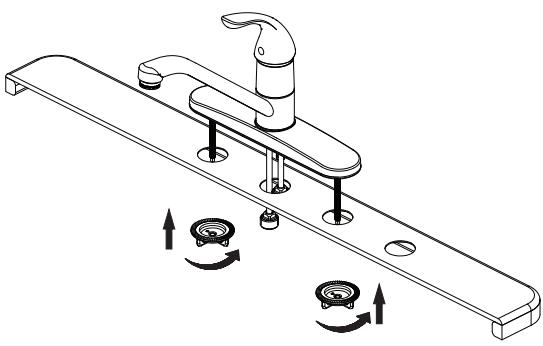
Shut off water supplies. Remove old faucet. Place faucet in position on sink. From under sink, thread mounting nuts onto faucet. Tighten mounting nut.
