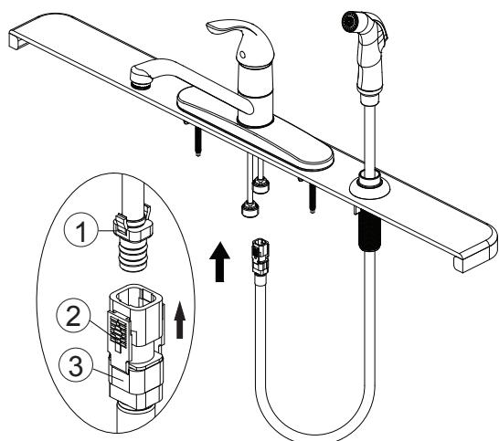
Insert spray hose down through the support and sink. Align tabs (1) and tabs (2) on quick connects (3). Push quick connector housing firmly upward and snap onto receiving tube tab. Pull down moderately to ensure connection has been made. If it is necessary to remove the quick connector, squeeze tabs on hose between index finger and thumb, then pull down to disconnect.
