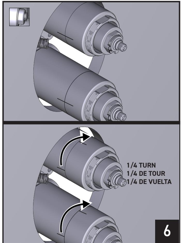
Do not overtighten cartridge nuts. Mark a line on the nut and body. With a wrench, rotate the nut closed 1/4 turn. Turn on the stops and check for leaks.
