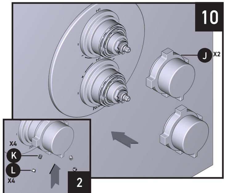
Install the Handles **(J)** (x2). Once the Handle is installed, insert and tighten the Handle Set Screws **(K)** (x4). Once the Handles are secured tightly, insert the Handle Plug Buttons **(L)** (x4).
