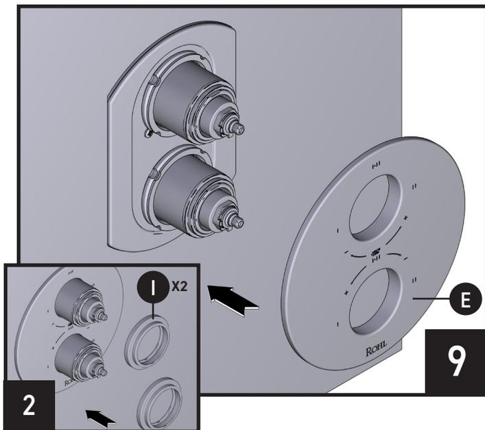
Install the Wall Plate **(E)** onto the Mounting Bracket Assembly. Once the Wall Plate is installed, install the Rosettes **(I)** (x2).
