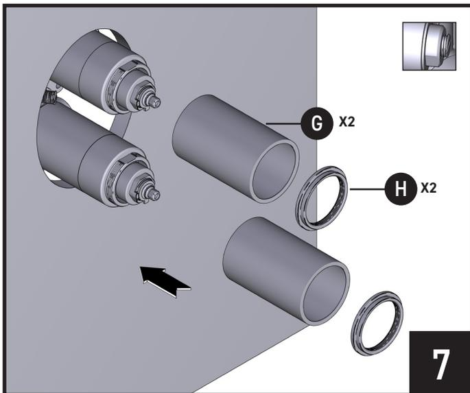
Install Decorative Sleeves **(G)** (x2) and Retaining Nuts **(H)** (x2). Tighten nuts, hand tight only.
