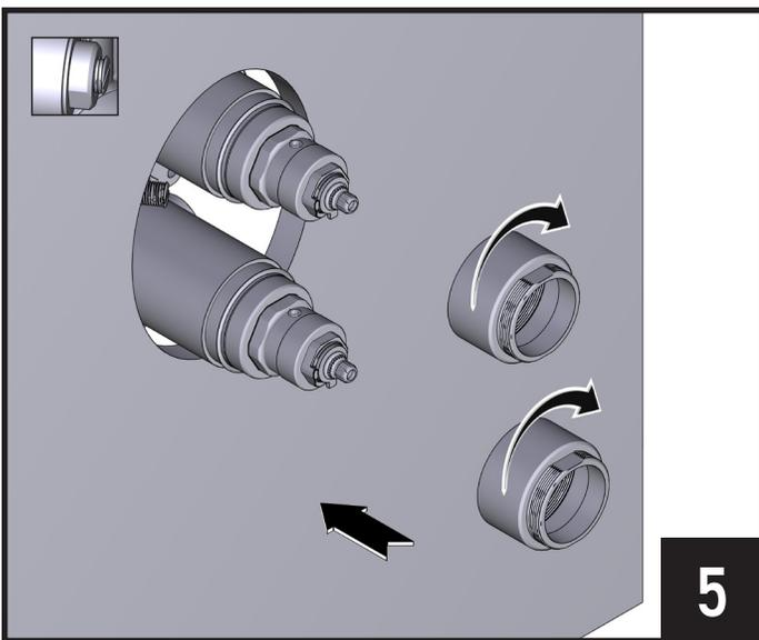
Slide Cartridge Nuts onto Cartridges and hand tighten.
