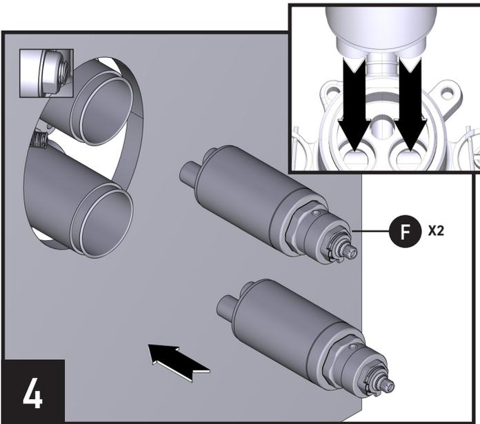
With stops in the close or vertical position, install Cartridges **(F)** (x2) into the Valve Assembly. Red inlet will be on the left, blue inlet will be on the right. Ensure that the ends of the Cartridges are installed correctly. Red marking on the Cartridges to be installed on the hot water line. Blue marking on the Cartridges to be installed on the cold water line.
