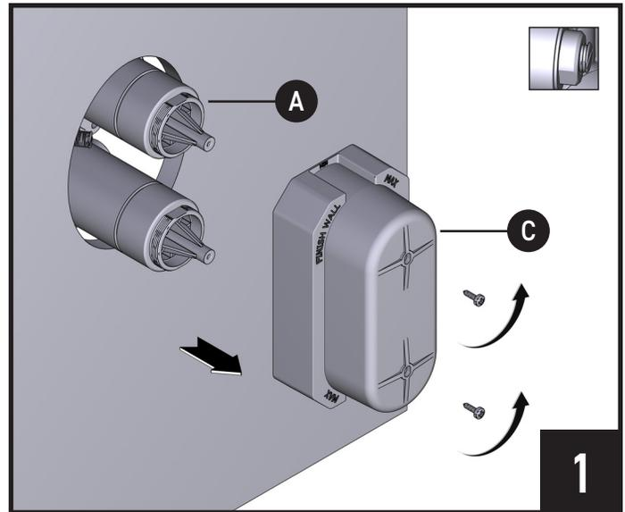
Remove Valve Cover and Plaster Ground **(C)** from existing Valve Assembly **(A)**.
