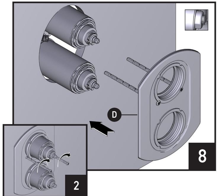
Install the Mounting Bracket Assembly **(D)** and secure with Mounting Bracket Assembly Screws (x2). Shorten the screws as needed. Apply sealant to the edges.
