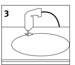
3. Using a saber saw, cut inside of the cutout line. Trial fit to check for proper fit.
