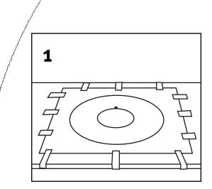
1. Select the bowl template that applies to the installation that you desire. Cut out the inside of the template. Locate the template front to rear and right to left on the countertop. Make sure that the bowl location will not interfere with the cabinet below or the plumbing. Attach the template to the countertop with masking tape and draw a pencil line around the inside of the template.
