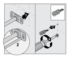
6b) **413TP Stud Option:** Place mounting brackets into desired position. Using brackets as a guide, carefully drill 3/16" holes into wall.
