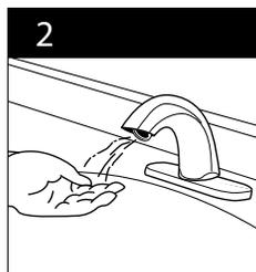
By placing your hands under the faucet, a sensor beam path is broken, causing the water to turn on.
