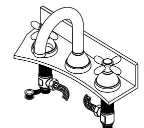
7. Connect water supply tube to the valve body. Use adapter if necessary.
