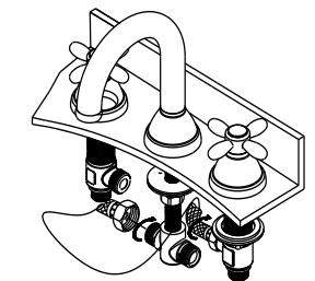
6. Apply pipe tape onto the threads of valve body adapter before connecting water supply tube.
