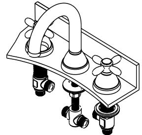
5. Connect the two flex hoses to the spout adapter. Make sure the right side hose connects to the left side of the spout adaptor and the left side hose connects to the right side of the spout adaptor.
