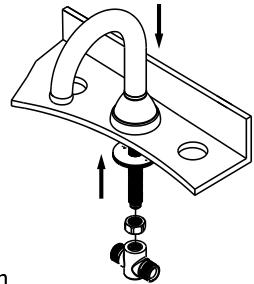
2. Disassemble the handle assembly by unscrewing the cap, screw, and canopy. Remove the top nut from the valve.
