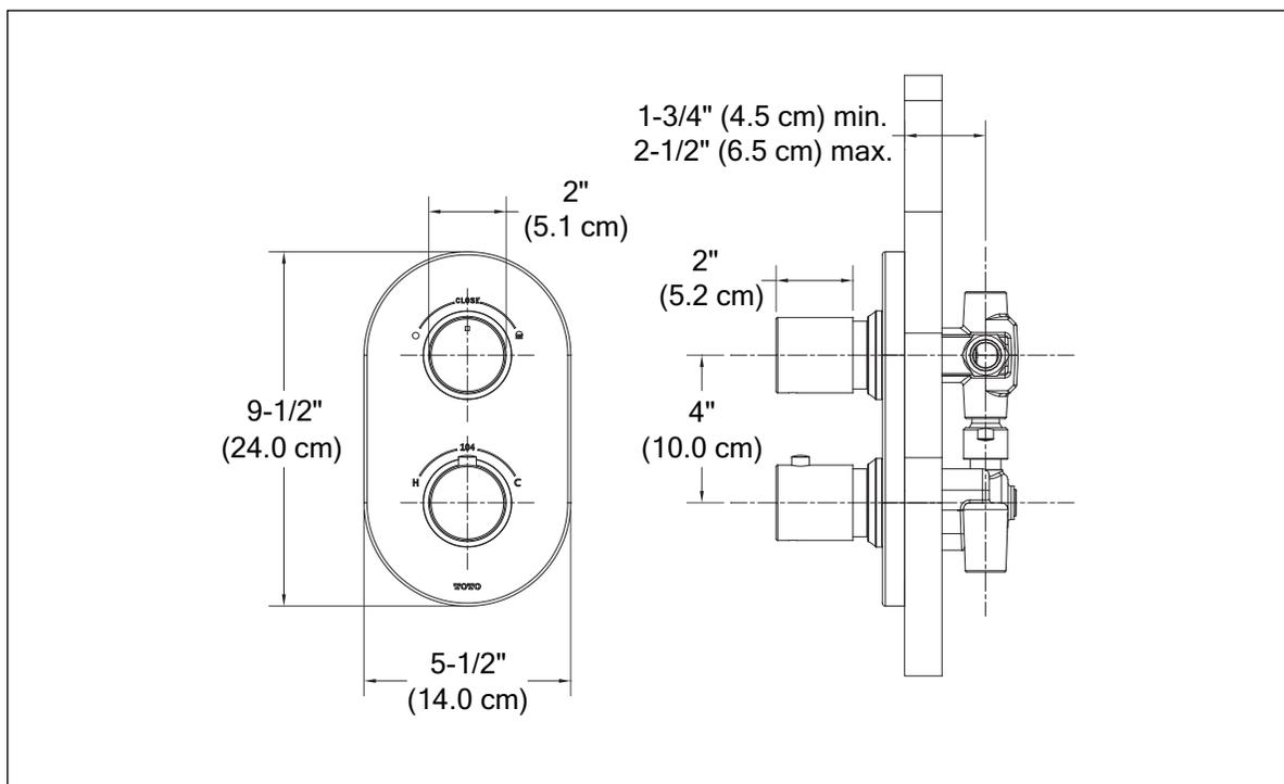
TS794D - Nexus® Thermostatic Mixing Valve Trim with Dual Volume Control
