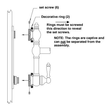
At this point, replace and tighten the lower three set screws and the upper three set screws using the 3/32" hex wrench provided in your installation kit. DO NOT OVERTIGHTEN THE SET SCREWS. Snug tight and firm is all you need. Once all six set screws are in place, thread the decorative upper and lower rings back onto the mounting bases to conceal the threads and the set screws. Hand tighten only, do not use a wrench.
