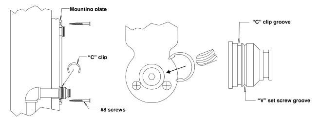
5. **ATTACH THE POTFILLER TO THE MOUNTING PLATE** - Your potfiller comes pre-assembled. Once the mounting plate is secure on the wall you are ready to attach the potfiller assembly. The upper and lower mounting bases on the potfiller have threaded decorative rings to hide the mounting set screws. Unscrew the upper and lower rings **away** from the mounting surface to reveal the
