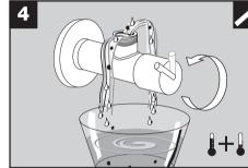
Before connecting supply lines to the water valves, flush each water valve to remove dirt and particles that can affect the functioning of the faucet and void warranty.
