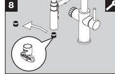
Remove aerator for standard water (14) with special key (15).
