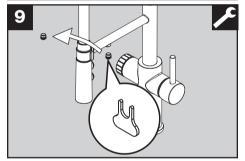
Also remove aerator for filtered water (10) with special key (11).
