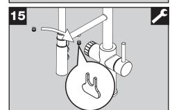
Reinstall the aerator for filtered water.
