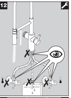
Double check all connections for leaks.
