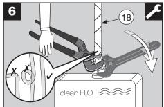
Connect supply line for filtered water (18) to water filter.
