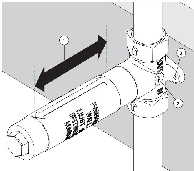
Install valve so the finished wall will be between the lines (1) indicated on the plasterguard. Make sure the water flows in the direction of the arrow (2) and that rough is level in the vertical and horizontal directions. Secure volume control using two mounting holes (3).
