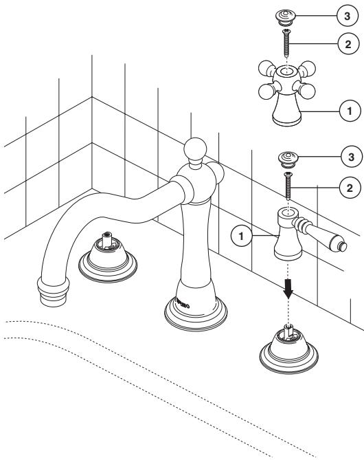
Install handle (1) onto valve stem. Secure with screw (2) and snap on handle button (3) which comes in the handle kit. If either handle does not rotate in the correct direction, do the following:
