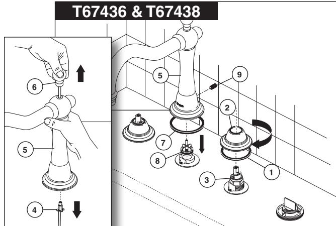
**NOTE:** The deck and valve rough-in must be finished before installing the trim kit.
